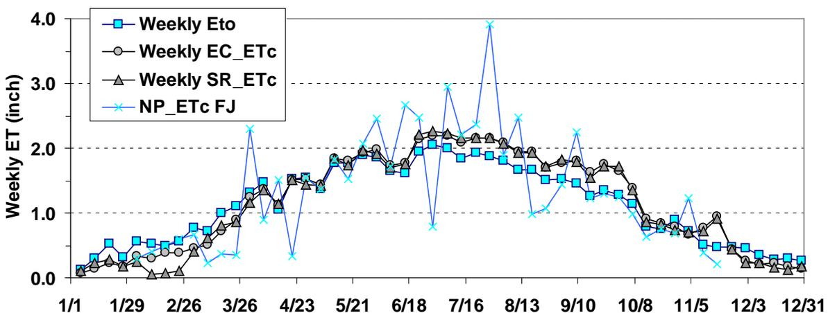
**Figure 1.** Weekly Fanjet ET from eddy covariance (EC), surface renewal (SR) and neutron probe soil moisture depletion/applied water (NP) compared to the Belridge CIMIS ETo for 2009.
