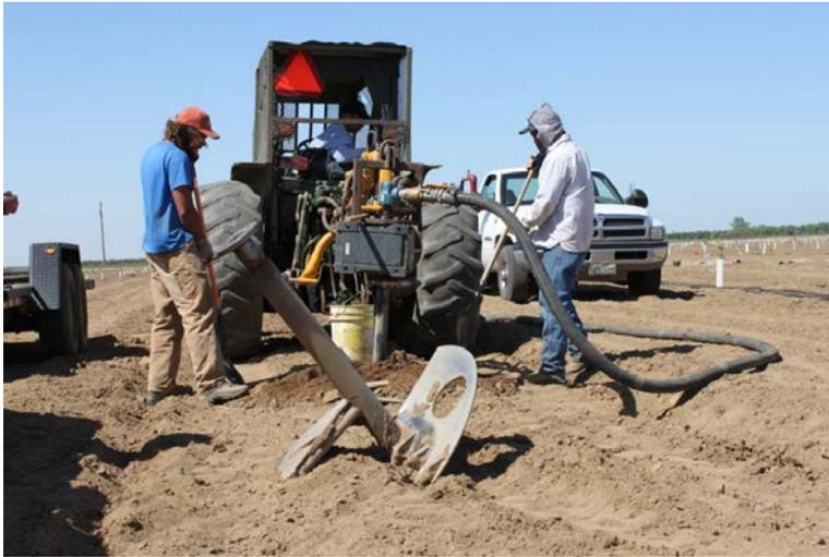
**Figure 1.** Redesigned steam-injection auger for treating almond tree planting sites. A 24-inch diameter auger (in use) and a 36 inch auger (foreground) were tested in trials near Delhi, and Wasco in 2011 and Livingston and Atwater in early 2012. Orchard performance will be monitored during the 2012 and 2013 growing seasons.
