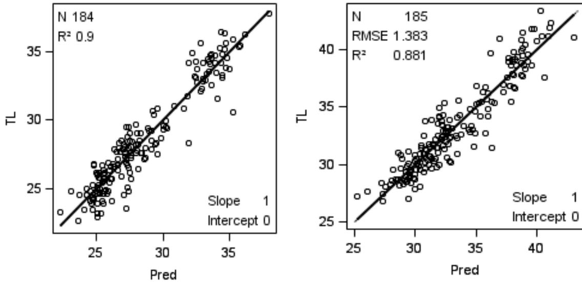
**Figure 5.** Multiple linear regression data comparing predicted (Pred) to measured leaf temperature (TL) using the new sensor suite for (a) shaded and (b) sunlit almond leaves.
