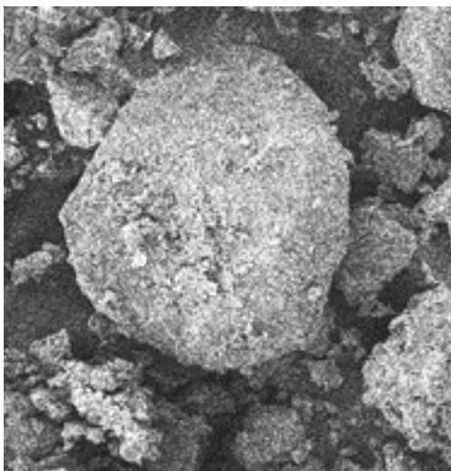
**Figure 4.** Scanning electron microscope image of collected particles.
