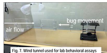
Fig. 7. Wind tunnel used for lab behavioral assays
